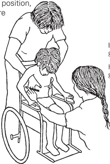
4. First, build in the guides in a temporary way.
