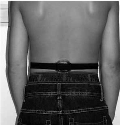
Figure 1. Example of an accelerometer and how it is attached to the body.
